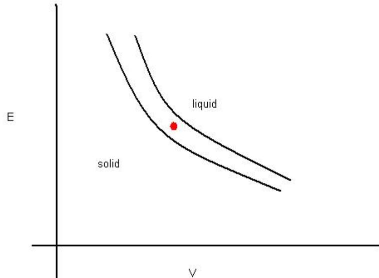
NVE ensemble: for fixed  $V$ , if  $E$  is between solid and liquid values, simulation will give coexisting solid and liquid
