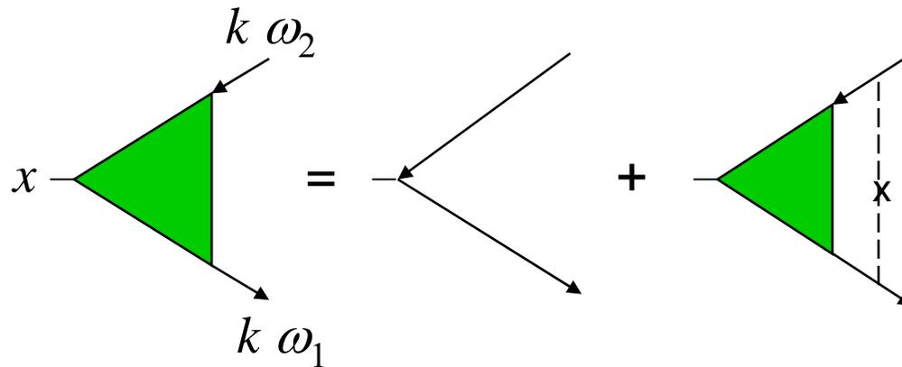
$$\Gamma_x(\vec{k}, \omega_1, \omega_2) = \tau_3 \sigma_x + \frac{1}{V^2} \sum_{\vec{k}'} \langle V_i(\vec{k} - \vec{k}') G(\vec{k}', \omega_1) \Gamma_x(\vec{k}', \omega_1, \omega_2) G(\vec{k}', \omega_2) V_i(\vec{k}' - \vec{k}) \rangle,$$
