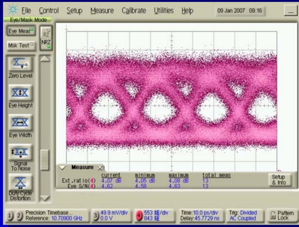
Eye Diagram Under 40 Gb/s NRZ Pseudo-Random Bit Sequence Modulation ( $V_{p-p} = 2$  V)
