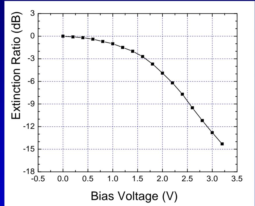
Static Extinction Ratio: 13 dB@-3V
