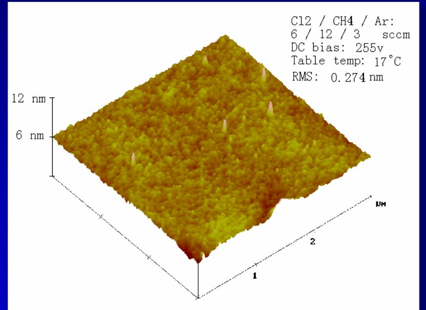
Surface Morphology Measured by AFM
