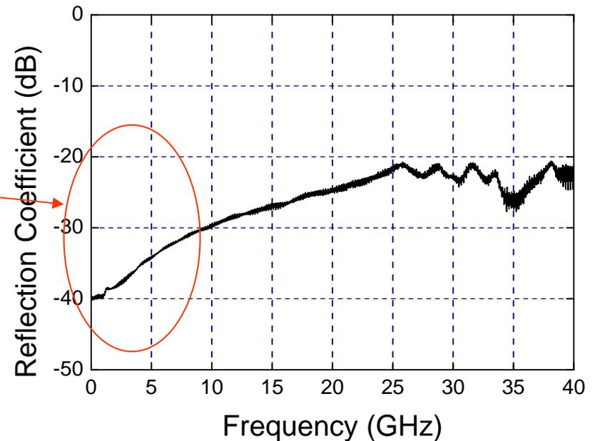
Microwave Reflection of  $\text{Al}_2\text{O}_3$
