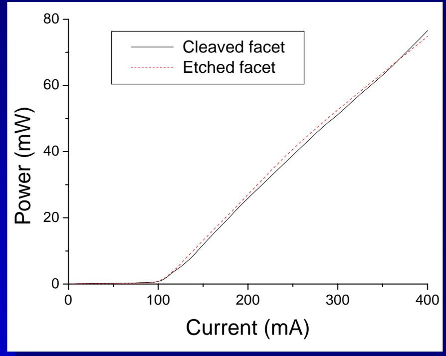
I-L Curves of Lasers with Cleaved
