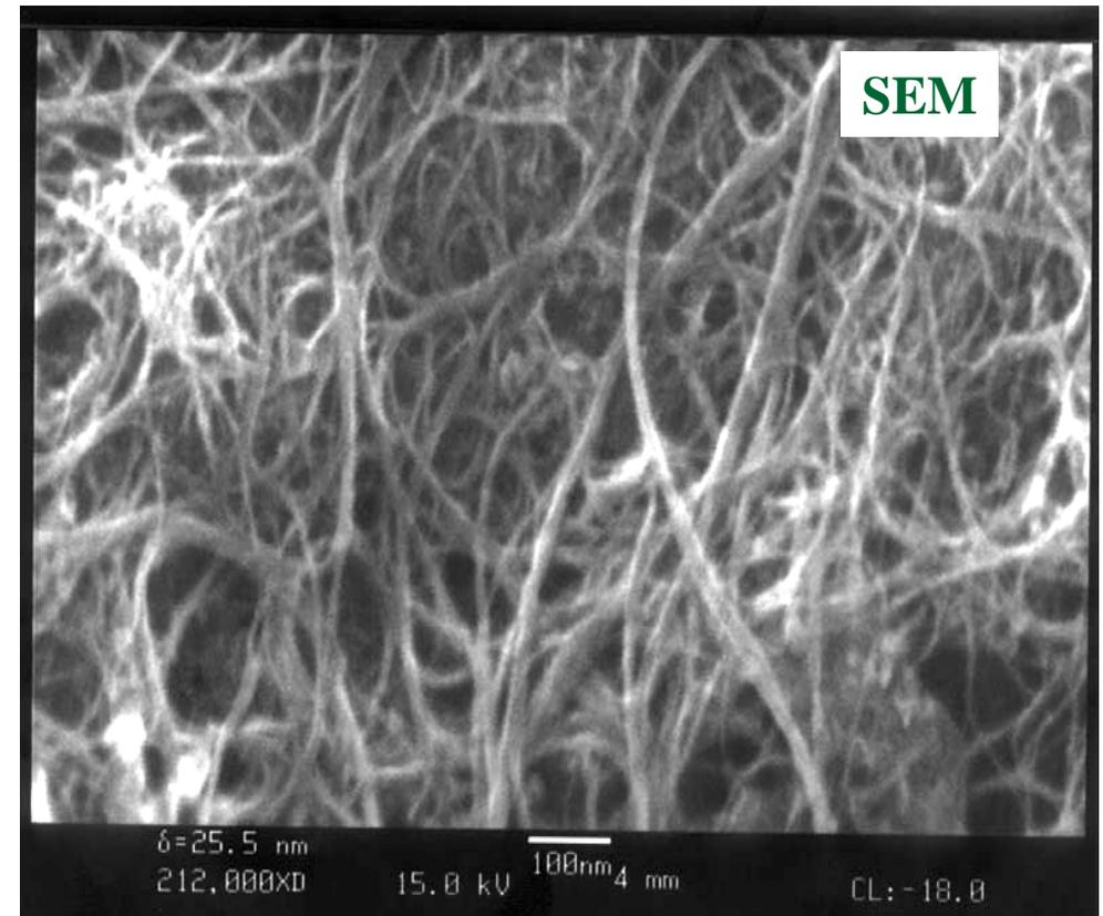
**Support: MgO; Catalysts: Fe; Carbon Source:  $\text{CH}_4$**
