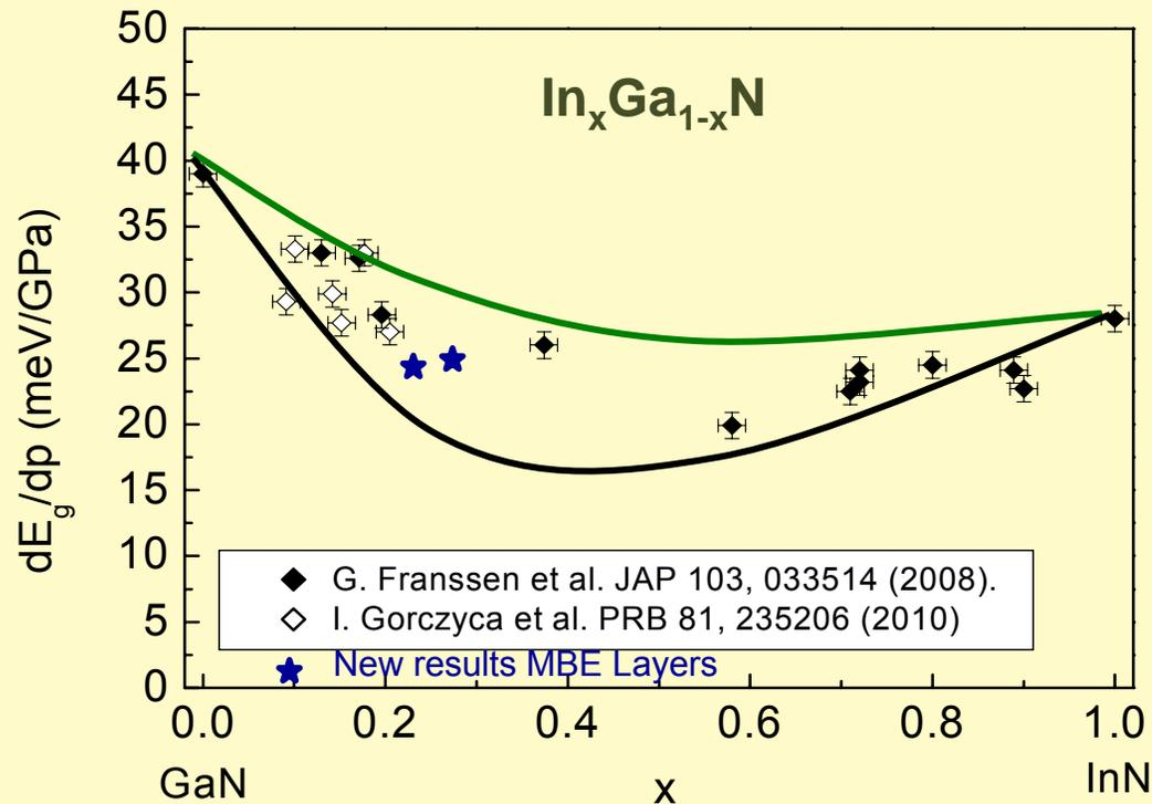
1. Significant bowing of  $dE_g/dp$  vs.  $x$  obtained by calculations with much more pronounced effect for clustered In-distribution
