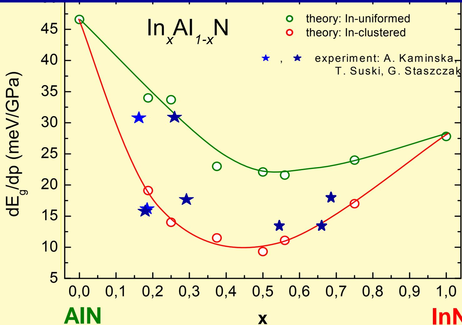
1. Drastic bowing  $dE_g/dp$  vs.  $x$  obtained by calculations with much more pronounced effect for clustered In-distribution.
