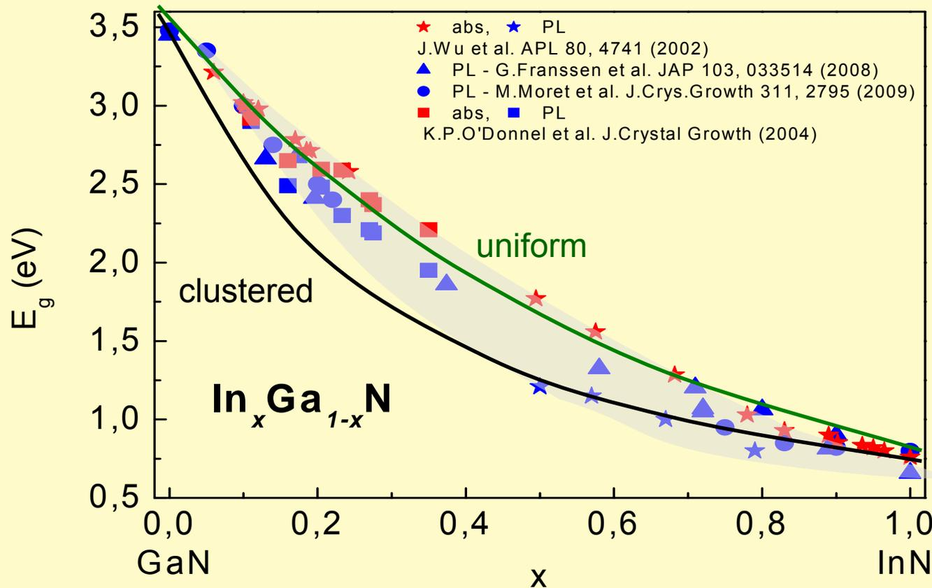
1. Significant bowing of  $E_g$  vs.  $x$  obtained by calculations with much more pronounced effect for clustered In-distribution
