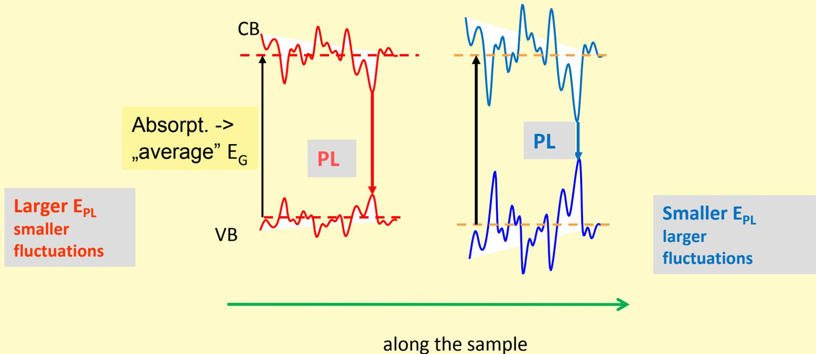
Our hypothesis: Fluctuations correspond to local In-segregation, we simulate it by first principle calculations
