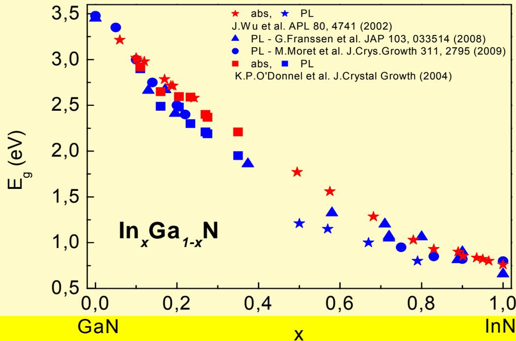
1. Large dispersion of data and significant bowing of  $E_g$  vs.  $x$  clearly seen
