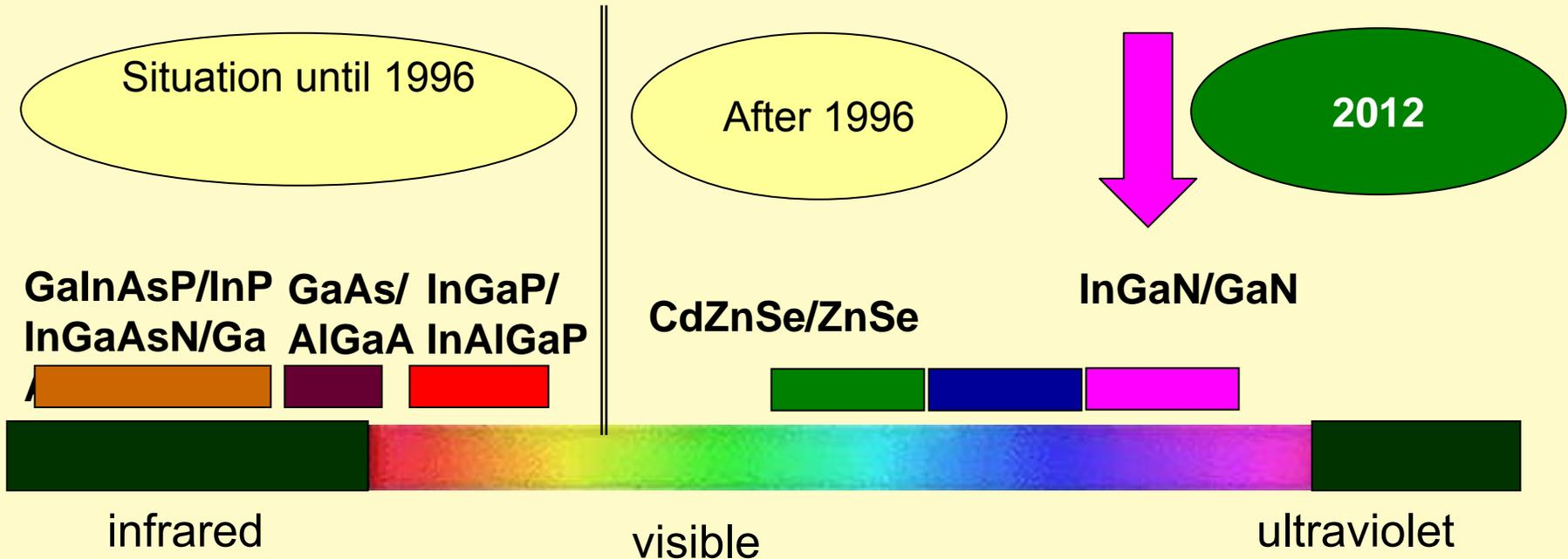
Period 1980-1995 characterized by intensive search for semiconductors enabling the laser action in the spectral range from yellow (600nm) up to UV (400nm)
