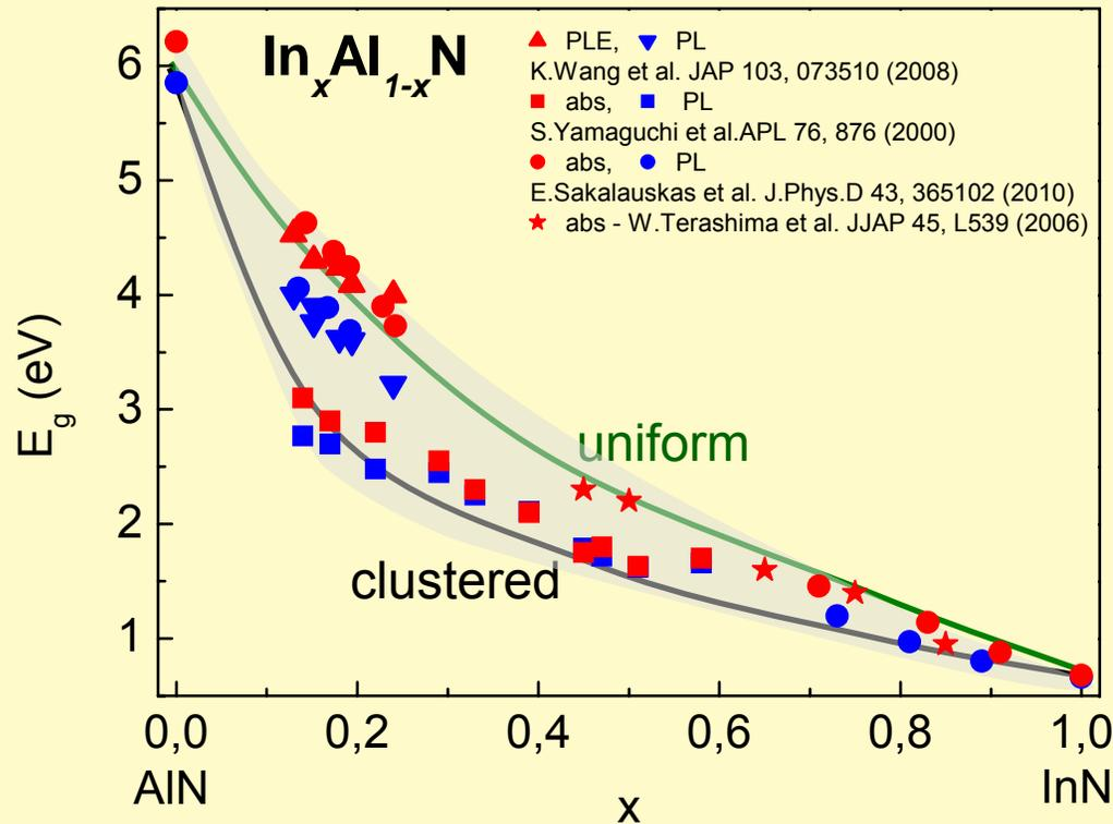
1. For  $\text{In}_x\text{Al}_{1-x}\text{N}$  - huge bowing of  $E_g$  vs.  $x$  obtained by calculations with much more pronounced effect for clustered In-distribution
