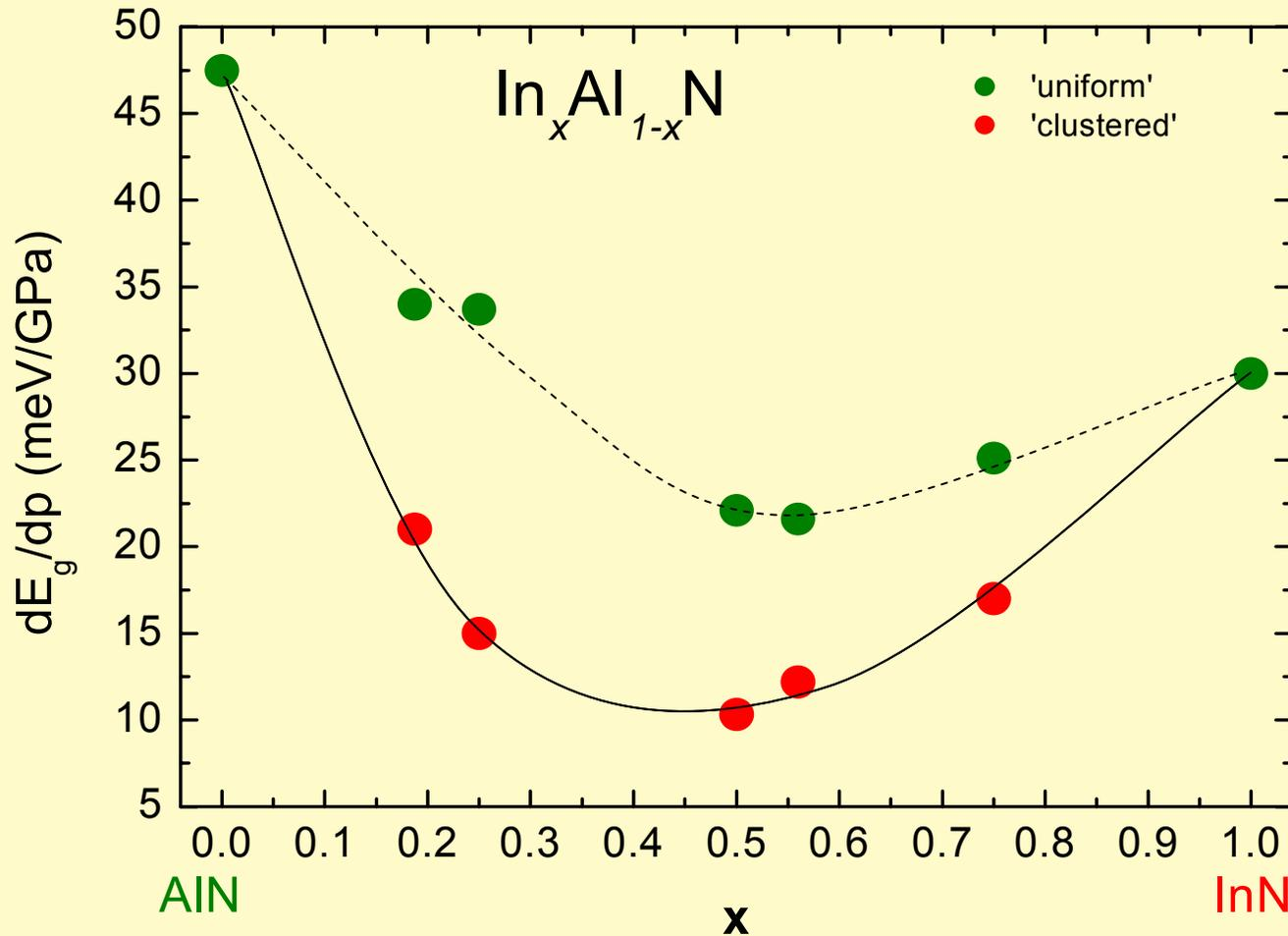
Predicted magnitude of pressure coefficient for clustered case much lower than for binary compounds. A chance for verification.
