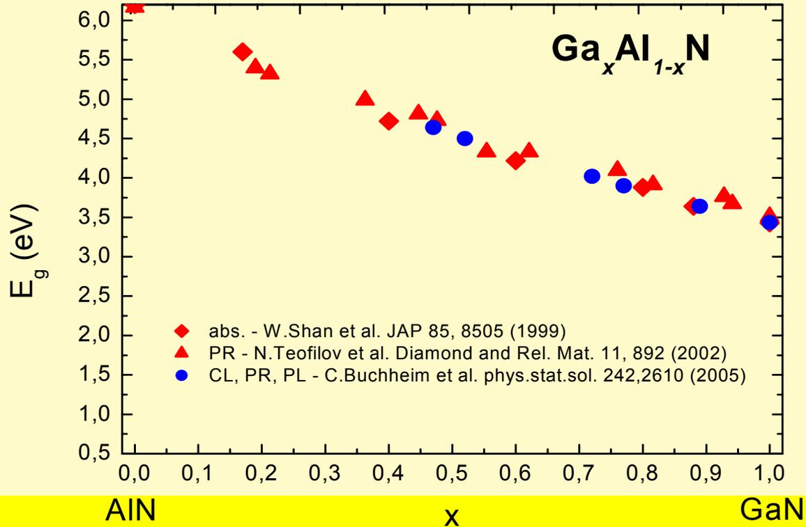
1. Small dispersion of data; almost linear dependence of  $E_g$  vs.  $x$
