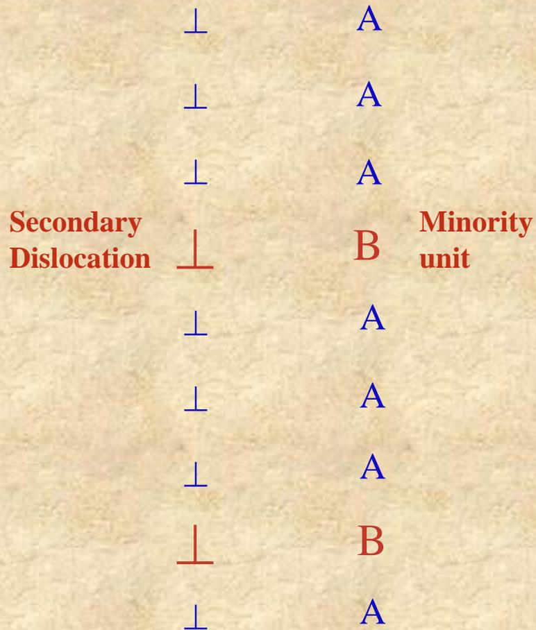
Each minority unit **B** is the core of a secondary dislocation with a DSC Burgers vector of the delimiting GB composed of **A** units.
